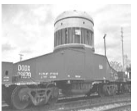
An upright DOE M-140 that carries waste shipboard reactor fuel to Idaho. This is the deadliest nuclear waste because it is left in Navy reactors far longer than fuel in commercial ones.
